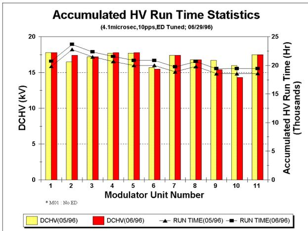
Fig.1: Accumulated run time of klystrons.
