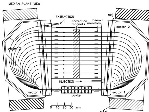
Figure 1: The 10–75 MeV Racetrack Microtron Eindhoven.
