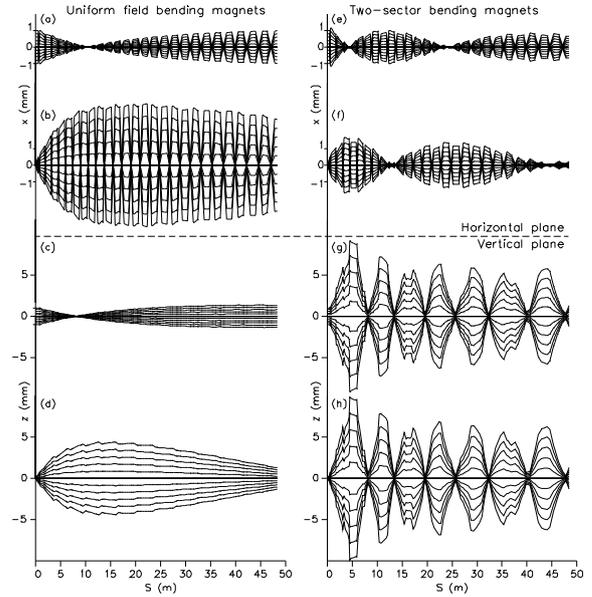
Figure 3: Trajectories in the horizontal and vertical plane for a parallel beam and for a divergent beam at injection. Homogeneous option: (a)  $x_0 = -1..+1$  mm,  $x'_0 = 0$ , (b)  $x_0 = 0$ ,  $x'_0 = -1..+1$  mrad, (c)  $z_0 = -1..+1$  mm,  $z'_0 = 0$ , (d)  $z_0 = 0$ ,  $z'_0 = -1..+1$  mrad. Two-sector option: (e)  $x_0 = -1..+1$  mm,  $x'_0 = 0$ , (f)  $x_0 = 0$ ,  $x'_0 = -1..+1$  mrad, (g)  $z_0 = -1..+1$  mm,  $z'_0 = 0$ , (h)  $z_0 = 0$ ,  $z'_0 = -1..+1$  mrad [2].
