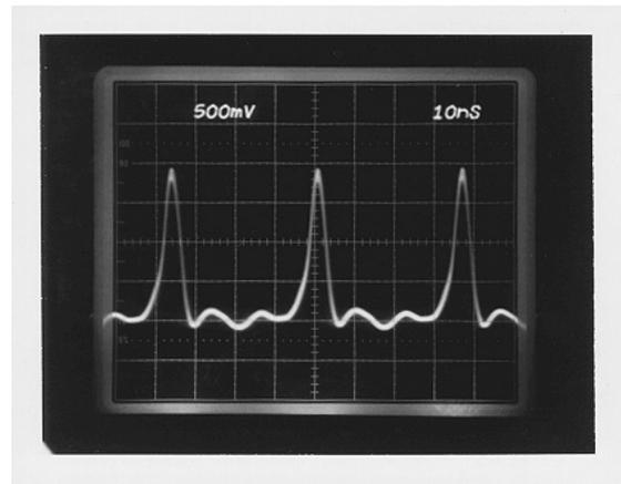
Fig. 4: Bunch current at RFQ output. The scale is 10 mA/div. vertically and 10 ns/div. horizontally.
