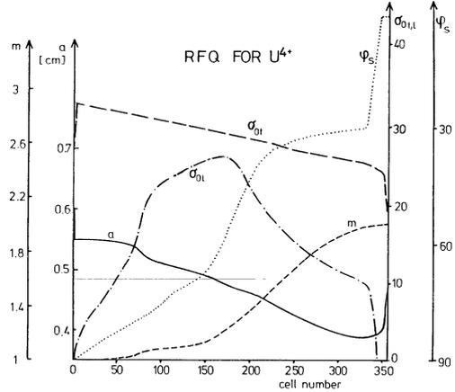
Fig. 3 RFQ parameters for the HSI-RFQ.
