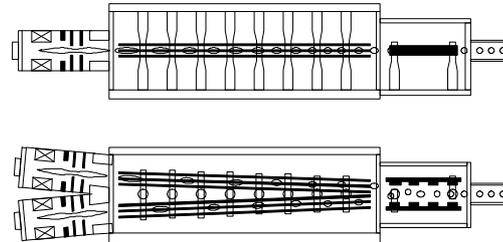
Fig. 5 Scheme of the two beam RFQ.
