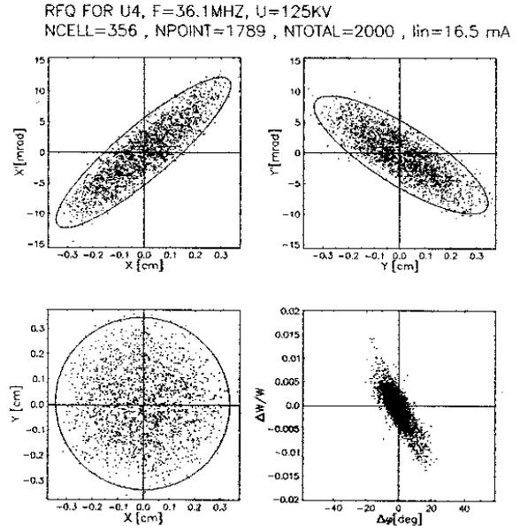
Fig. 4: Output distribution for a 16.5 mA input beam.
