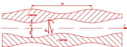
Fig. 1 Scheme of RFQ electrodes.
