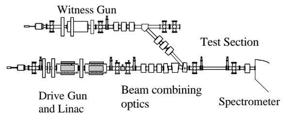
Figure 1. Schematic layout of the AWA facility.
