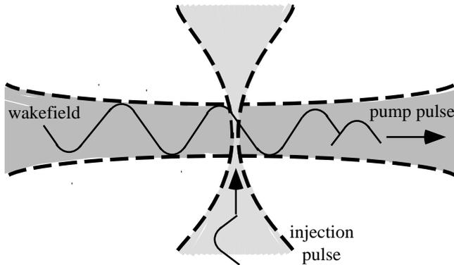
Figure 5. The LILAC concept: one pulse drives a wakefield and another injects electrons.
