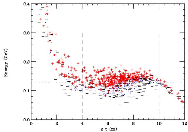
Figure 2: Energy vs ct of muons at end of decay channel with phase rotation; muons with polarization  $P > \frac{1}{3}$ ,  $-\frac{1}{3} < P < \frac{1}{3}$ , and  $P < -\frac{1}{3}$  are marked by the symbols '+', '.', and '-' respectively.
