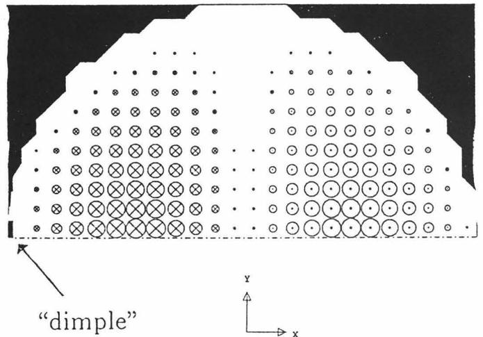
Figure 3: Geometry which has been used to calculate the center shift of the TM11 like dipole mode in a single cell due to a single deformation with a diameter of 6 mm and a height of 1 mm.
