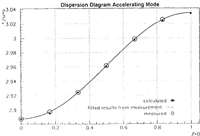
figure 4: dispersion diagram of the accelerating mode passband including the frequencies calculated by mafias.
