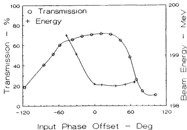
Fig. 1. The output energy of the linac, and linac transmission, as a function of the phase of the injected beam relative to the linac rf. The absolute value of the phase shown is arbitrary.
