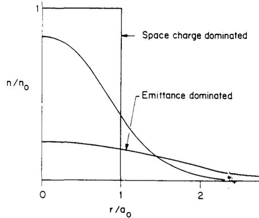
Sketch showing transverse profiles of a matched distribution with thermal transverse velocities and finite emittance in a uniform channel with linear focusing. Transition from a square to a gaussian density distribution occurs as  $\sigma/\sigma_0$  varies from zero to unity. In the intermediate regime  $K \approx e^2/a^2$ , or the Debye length  $\lambda_D \approx a$ .
