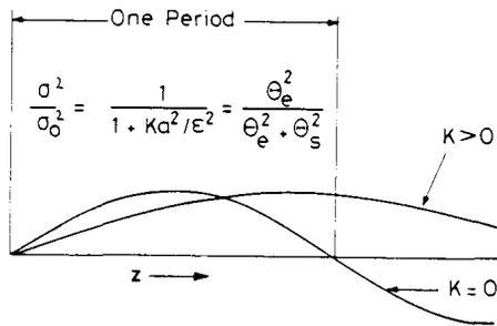
Illustration of the meaning of  $\sigma/\sigma_0$  in a K-V beam with smooth approximation. This may be expressed either in terms on the perveance and emittance, the characteristic space-charge and emittance angles, or the plasma frequency and betatron frequencies in the absence of space charge; this may be seen from Eq.4.
