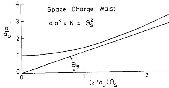
Waists arising from space-charge and emittance. The envelope equations are found from Eq.3 with  $a=b$ , including only the two relevant terms.
