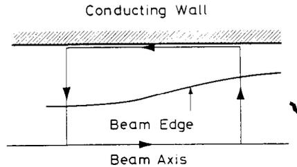
Diagram to illustrate the transition from longitudinal to transverse configuration in a beam that changes its transverse configuration.  $\int E dl$  round the rectangle is zero and since the contribution along the conducting wall is zero, the value along the axis is equal to the difference of the numerically unequal radial contributions.
