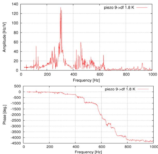
Figure 2: PZT voltage to detuning transfer function., amplitude (top) and phase (bottom).
