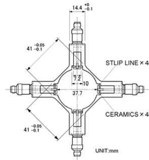
Figure 2: Schematic of beam position monitor in MEBT1.
