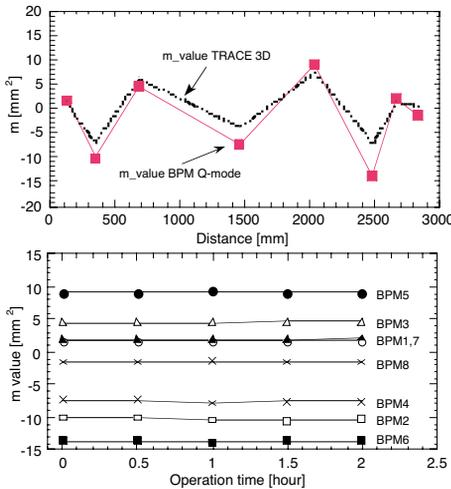
Figure 8: Experimental and calculated results of beam size term (a). Sufficient reliability of beam size measurement during the practical long time period was also confirmed (b).
