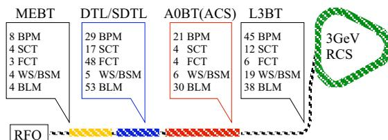
Figure 1: Designed beam monitor system in the J-PARC linac.
