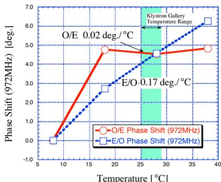
Figure 5: Temperature characteristics of the new O/O and O/E.
