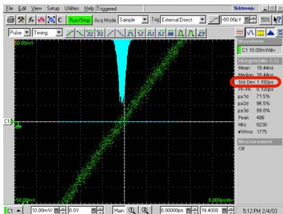
Figure 4: E/O transfer jitter measured by using a TDS8000B. Because the jitter of the measurement system is about 0.8 ps, the net jitter is  $\sqrt{(1.2^2 - 0.8^2)} = 0.9$  ps.
