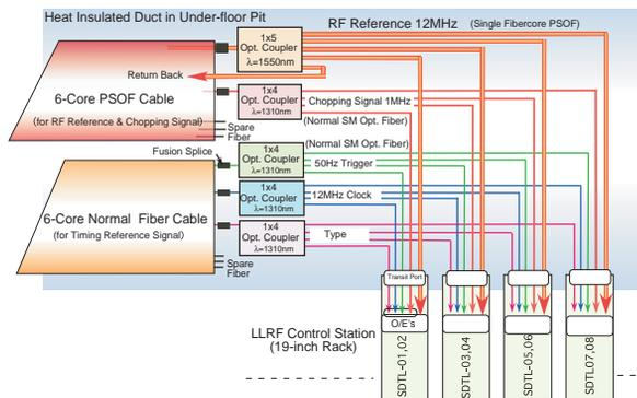
Figure 7: Providing RF and timing reference to each control station.
