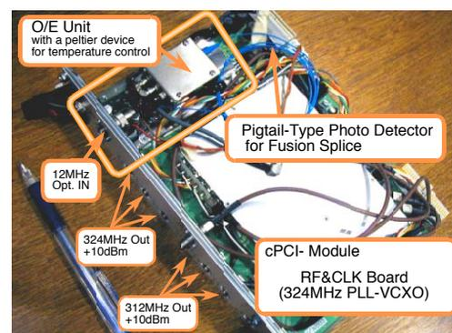
Figure 3: New O/E with a temperature stabilizer.
