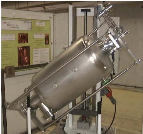
Figure 5: Stainless steel frame and bracing rods as cavity stiffness.
