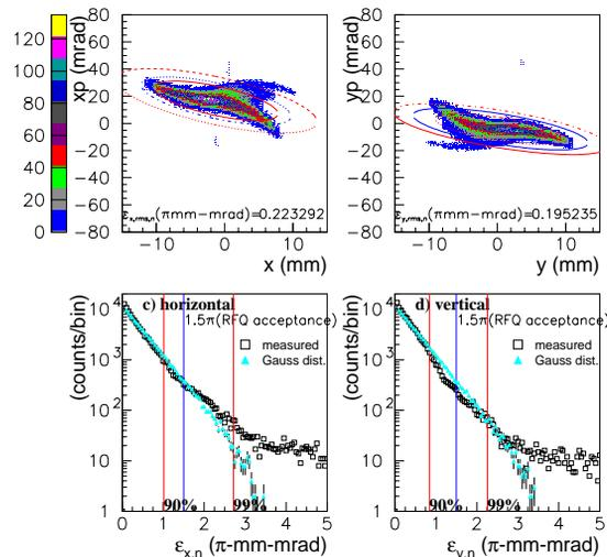
Figure 1: Measured emittances of the LEBT. The left-top and right-top show the phase space plots in the  $x-x'$  and  $y-y'$  planes, respectively. The ellipses are 90%,  $1.5\pi$  mm-mrad (design acceptance of the RFQ) and 99% emittances. The bottom figures represent the beam current in the slices of the ellipses. The beam current is normalized to 100000. Open squares show the experimental result and closed triangles represent the distribution used for the simulation.
