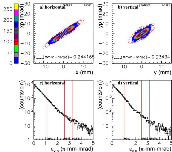
Figure 6: Simulation result at the MEBT exit using with the distribution obtained with PARMTEQM.
