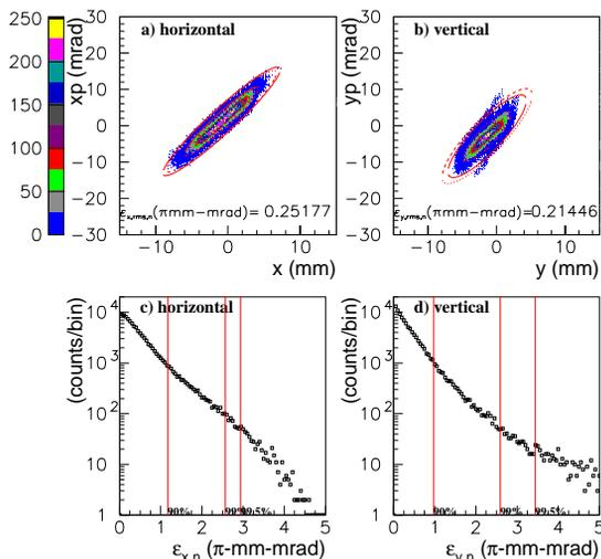
Figure 5: Measured emittances at the MEBT exit.
