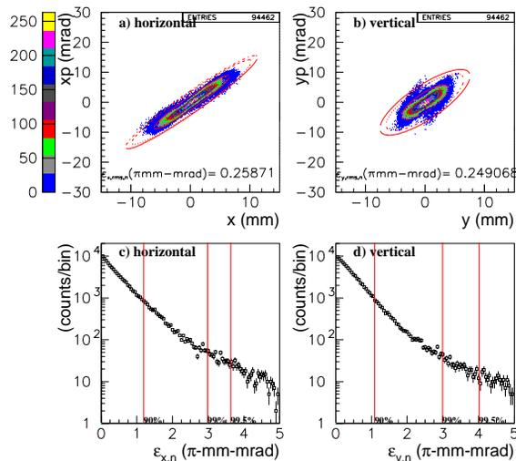
Figure 7: Simulation result at the MEBT exit using with the distribution obtained with TOUTATIS.
