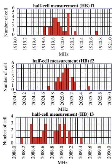
Figure 5: Frequency distribution of 28 half-cells (high-beta model)
