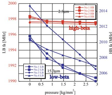
Figure 3: Effect of flatness on frequency shift
