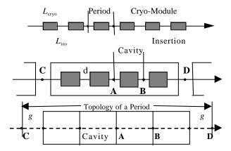
Figure 1: Configuration of a Proton SCL Accelerator.
