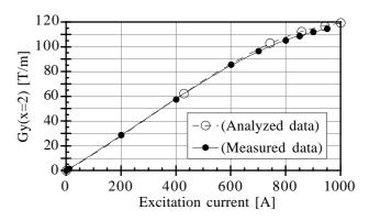
Figure 3: Comparison of excitation-current dependences on magnetic field gradient for measured data and 3-D analyzed data using MAFIA.
