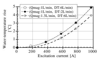
Figure 5: Excitation-current dependences on increase in the water-temperature of the electroformed coil.
