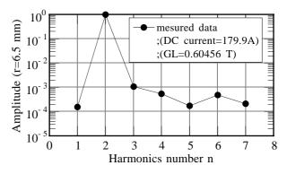
Figure 4: The higher-order multipole components in the center of the magnetic field.
