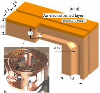
Figure 1: A detail of a corner part of the electroformed hollow coil.
