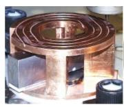
Fig. 2e: Separation of the coils by end mill.
