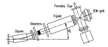
Figure 3: Layout of the measurement line.
