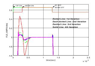
Figure 1 Field Amplitude with PI Controller plus Iterative Learning Controller (PI+ILC) .
