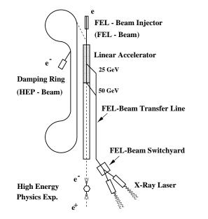
Figure 1: The  $e^-$  linear accelerator of the TESLA linear collider with integrated x-ray laser facility.
