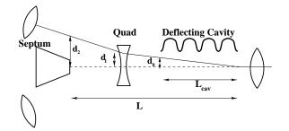
Figure 5: Fast FEL-Beam Splitter. The kick due to the defecting mode is enhanced by a defocusing quadrupole magnet.
