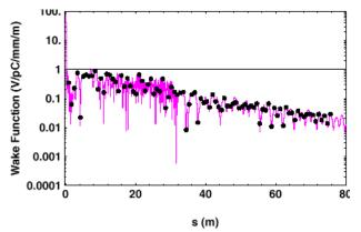
Figure 5: Envelope of wake function for RDDS1 excluding external loading
