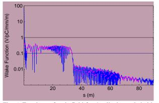
Fig. 6: Envelope of wakefield for 4 cells decoupled either end of structure and  $Q\sim36$  for the last cell
