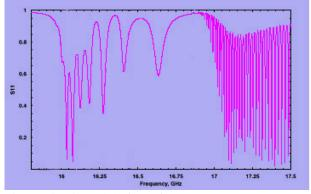
Fig. 2: Circuit model of S<sub>11</sub> of output port
