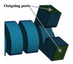
Fig 1: Fundamental four-port coupler
