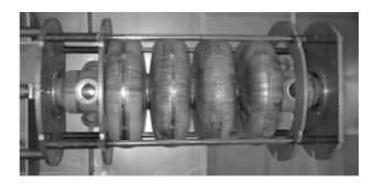
Figure 5: The prototype 4-cell  $\beta$ =0.7 cavity
