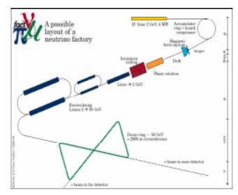
Figure 3: Possible layout of a Neutrino Factory
