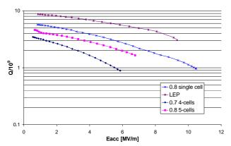
Figure 6: Q vs. gradient of the sputtered-Nb cavities
