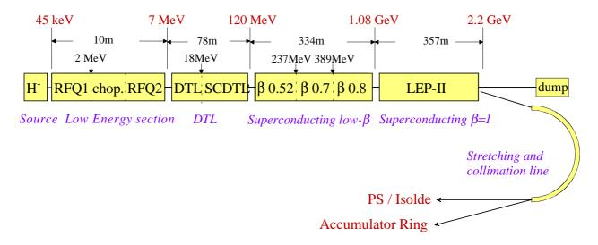
Figure 4: Layout of the SPL H linac
