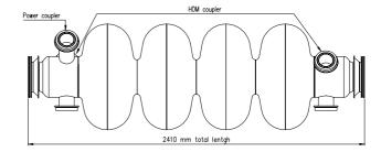
Figure 1: The LEP-2 accelerating cavity
