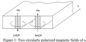
$TE_{01}$  mode in a rectangular waveguide.
