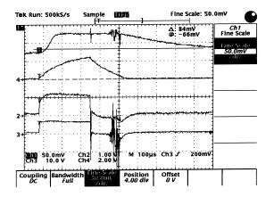
Figure 7. Measured phase shifter response. 1=phase detector output, 2=pulse transformer input voltage (x1000 probe), 3=pulse transformer output voltage, 4=phase shifter bias current (1 V for 100 A).
