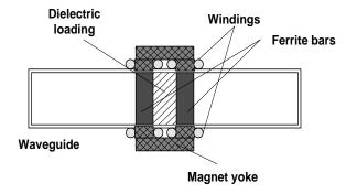
Figure 2. Cross section of a waveguide phase shifter.
