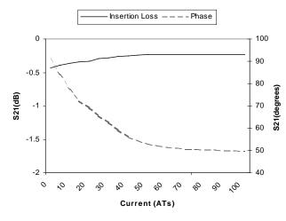
Figure 6. Measured phase shift and insertion loss vs. bias current.
