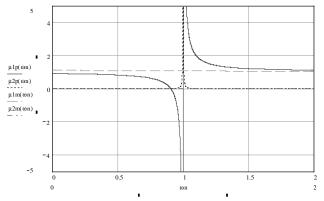
Figure 3. Complex permeability of a YIG material,  $4\pi M_s = 250$  Gauss,  $\Delta H_t = 4$  Oe,  $\omega_s = \omega_s/\omega$ .
