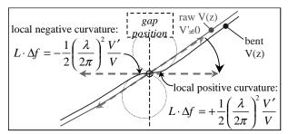
Fig. 4. Local bend of V(z) to get a horizontal tangent
