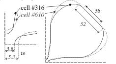
Fig. 1. RFQ cross-sections at two different locations.
