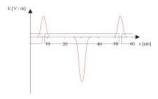
Figure 6: distribution of electric field along axis
