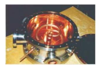
Figure 9: View into open splitring cavity
