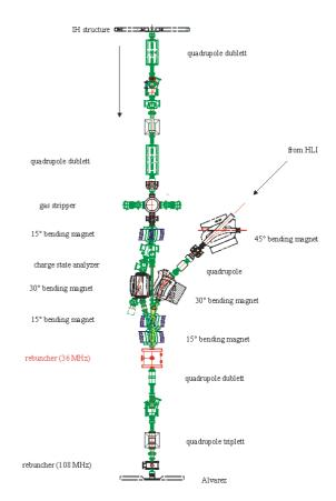
Figure 4: Stripper section of the UNILAC
