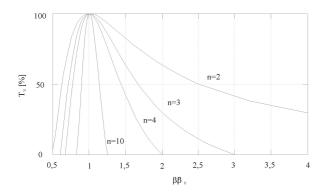
Figure 2: velocity depend term of the transittime factor
