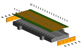
Figure 6: Exploded view of the 35-cm current structure assembly (courtesy of R.J. Roybal, LANSCE-1)
