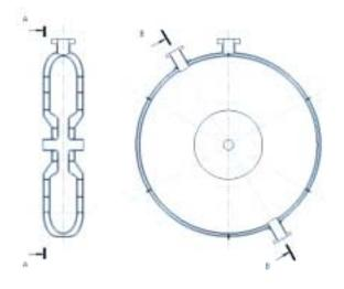
Fig.1 Mechanical design of the reentrant cavity.
