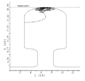
Fig.2. Example of the multipacting simulation program output (the horizontal axis is stretched in the picture). The circular contour, as well as the rectangular one, was causing high field multipacting levels.
