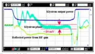
Figure 4: L3 Klystron phase – after adjustment of phase compensator.
