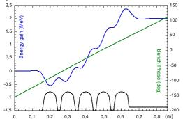
Figure 2: Energy gain and phase slippage along the  $\beta$ =0.50 cavity (G = 8.5 MV/m,  $E_{in}$  = 85 MeV,  $\varphi_b$  = -30°).
