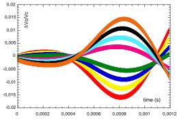
Figure 7: Amplitude of the 8 cavity voltages for the last group (with Lorentz forces only).
