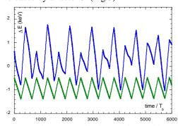
Figure 3: Bunch energy gain along - chopped beam pulse (bottom: single resonator model; top: multi-mode model).
