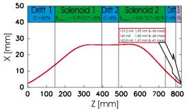
Figure 7: Schematic drawing of the magnetic LEBT for IFMIF including beam envelope for 140 mA.
