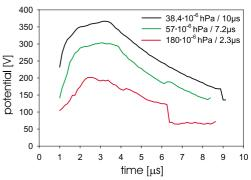
Fig. 6 : Development of the beam potential as a function of time for different residual gas pressures measured by time resolved residual gas ion energy spectrometry.
