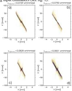
Figure 8: Simulation of beam transport for constant space charge ( $f_{noise} < 20$  kHz) using entrance emittances according to fig. 1.
