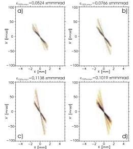
Fig. 4: Output emittances of the electrostatic LEBT gained by transport simulations using 3 different ion currents (a-c) and superposing them for time integration (d).
