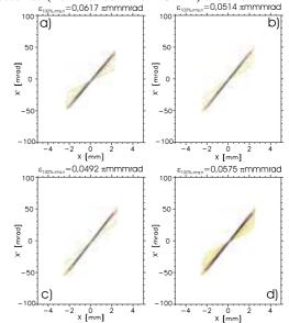
Fig. 2 : Emittances at the entrance of the LEBT system for varied extracted beam currents (a.) 137.2 mA, b.) 140 mA, c.) 142.8 mA, d.) time integrated (a+b+c)).
