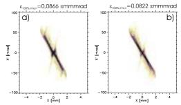
Figure 9 : Time integrated emittance gained from simulations of beam transport using entrance emittances according to fig.1(a)  $f_{noise} \approx 100$  kHz, b)  $f_{noise} \approx 500$  MHz).
