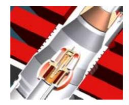
Fig. 3. Magnetron injection gun sectioned view
