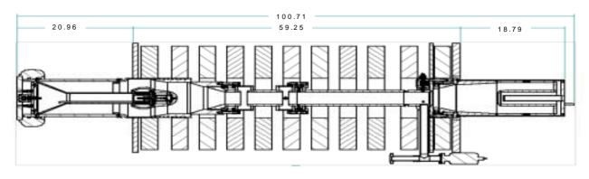
Fig. 4. Cross section of ABK beamstick with magnet coils
