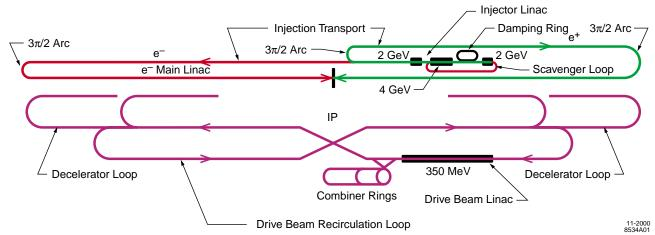
Figure 2: Schematic Layout of a Two-Beam Linear Collider with Recirculation and Central injector. The upper beam lines are for the main beam while the lower ones are for the drive beam. All long beam lines are in the same tunnel. The vertical scale is expanded for clarity. The injector linac sits beside the drive beam linac. View animation here.
