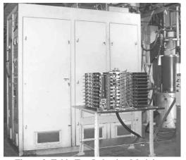
Figure 8. Table Top Induction Modulator
