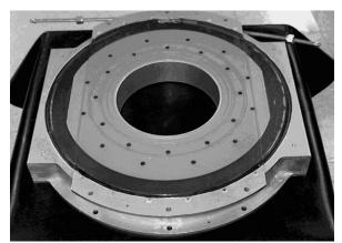
Figure 2. Metglas Core in case
