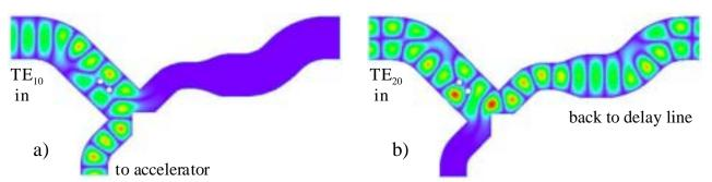
Figure 3: Extractor with simulated electric field plots illustrating a) extraction of the  $TE_{10}$  mode and b) passing the  $TE_{20}$  mode. For the latter, a "jog converter" attached to the through port after a width taper restores the mode and brings the port back in line with the delay line. Power flow is from the left port.
