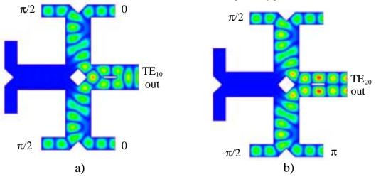
Figure 2: Example Cross Potent Launcher with simulated electric field plots illustrating launching a)  $TE_{10}$  and b)  $TE_{20}$  in the right overmoded rectangular port with the indicated relative phases for four equal amplitude inputs. Alternate phasings of the inputs send the power to either of the left ports.
