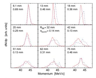
Figure 2: Measured (solid line) and calculated (dotted line) momentum spectra at the end of the beam line for different compressor settings  $R_{56}$ , with a bunch charge of 5 nC. The measured bunch lengths are also shown (lower values).
