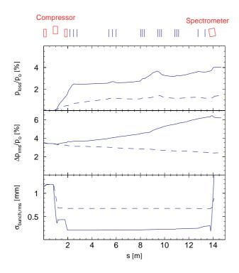
Figure 5: Evolution of the bunch length, the rms momentum spread and the momentum loss (from bottom to top) along the CTF II beam line as simulated with TraFiC<sup>4</sup>, for 10 nC. The results with two different setting of the chicane are shown, corresponding to  $R_{56} = 34$  mm (solid line) and  $R_{56} = 15$  mm (dashed line).
