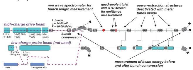
Figure 1: The CLIC Test Facility CTF II. The CSR experiments were performed in the drive beam line (upper part).
