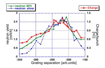
Figure 8: Electron and neutron yield versus compressor position.
