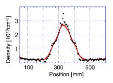
Figure 5: Extracted density profile obtained with the folded wave interferometer. The helium plasma was produced by laser ionization of the gasjet plume.
