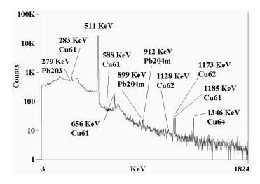
Figure 9: Example gamma ray spectrum from the nuclear activation measurements, showing the peaks corresponding to each isotope produced.
