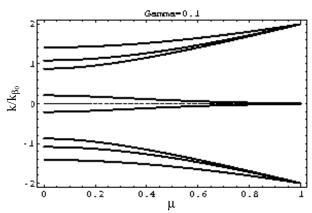
**Figure 1**. Mode frequency vs. tune depression for  $\Gamma$ =0.1. For  $\alpha$  < 1/27  $\cong$  0.037 all modes are real.
