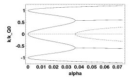
**Figure 2.** Frequency (in units of  $k_{00}$ ) of quadrupole and low frequency modes vs. parameter  $\alpha$  (see text). (Solid is real, dashed is imaginary). Note for  $\alpha > 1/27$  the low frequency quadrupole and low frequency merge, and an unstable mode appears.
