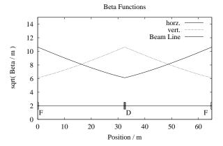
Figure 3: Standard FODO cell of the linac (60° phase advance). The square root of the horizontal (solid line) and vertical (dashed line) beta-function are shown versus the longitudinal position for the HEP beam.
