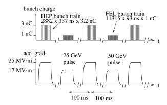
Figure 2: HEP and FEL beam pulse structure
