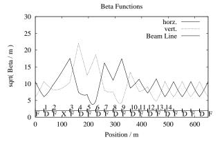
Figure 7: Simultaneous beam matching with a missing quad. The square root of the horizontal (solid line) and vertical (dashed line) beta-function of the HEP beam is shown.
