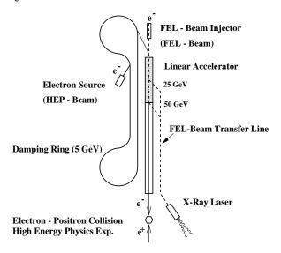
Figure 1: The e<sup>-</sup> linear accelerator of the TESLA linear collider with integrated x-ray laser facility.
