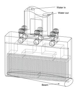
Figure 3: Chopper Target
