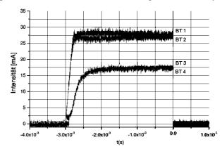
Fig. 4 Beam transformer signals along the beam line.
