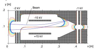
Fig. 3 Equipotential planes with voltages  $-10 \text{ V} \ge \text{U} \ge$  -100 V and deflected beam in the electrostatic chopper
