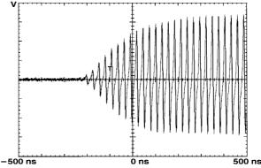
Fig. 7 Beam macropulse rise behind the RFQ
