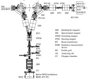
Fig. 1 Mechanical layout of the new LEBT
