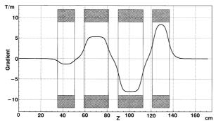
Fig. 6 Measured quadrupole quartet field distribution
