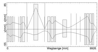
Fig. 2 Transverse envelope of a zero current beam
