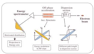
Figure 2 Transformation of longitudinal phase space distribution using the dispersion section and the off-phase accelerating structure.
