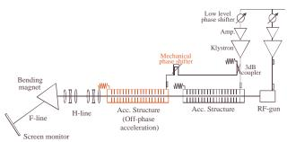
Figure 3 Layout of BNL-ATF beam line
