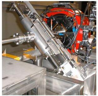
Fig.1: Wire scanner chamber in ATF extraction line.
