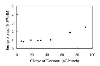
Figure 3: Electron charge dependence of the energy spread of the single-bunch beam.
