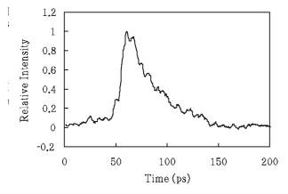
Figure 5: Time profile of the single-bunch beam measured with a streak camera at an electron charge of 73 nC/bunch.
