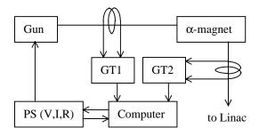
Fig. 1 Gun feedback control block diagram.
