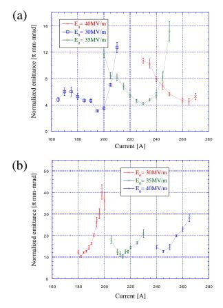
Figure 2. Measurement of the emittance at the exit of the 9cell for (a) 1nC and (b) 8nC versus current in the solenoids for three values of  $E_0$ .
