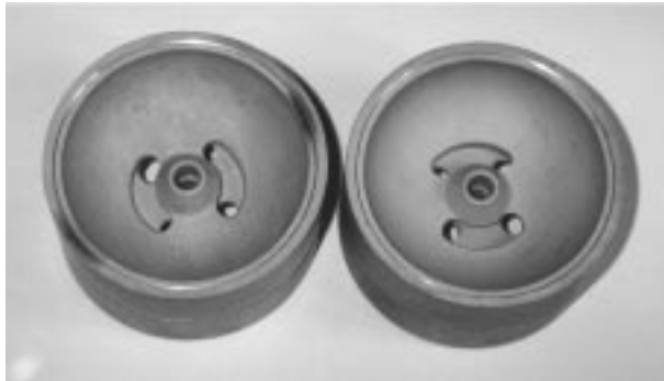
Figure 1. A general view of the S-band CDS \beta = 1.0 cold model, k_c = 22\% .
