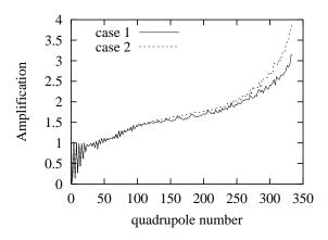
**Figure 5:** The maximum amplification of an initial beam jitter along the decelerator. The case of a rectangular current pulse (case 1) is compared to the one with a ramp in bunch number (case 2).
