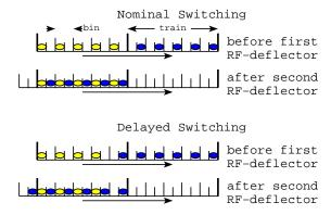
**Figure 2:** The scheme of delayed switching. In this example, each train contains 5 bins (an arbitray number chosen for better visibility). In the upper case the phase is switched at the nominal time, creating a rectangular pulse. In the lower case the phase switch is delayed to create a ramp.
