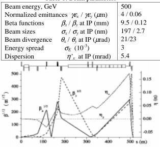
Figure 3: Optics of the new NLC Final Focus System showing horizontal and vertical betatron and dispersion functions similarly to Fig.1
