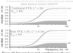
Figure 10: Integrated spectral contribution to the rms vertical beam offset at the IP from ground motion for the NLC-FFS and the new-FFS. The main contribution being from the final doublet (Ideal Optical Anchor OFF)
