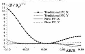
Figure 5: FD bandwidth of the Traditional and New NLC Final Focus. Normalized betatron functions at the final doublet versus energy offset  $\Delta E/E$ .
