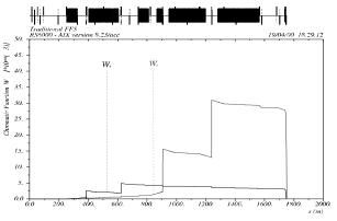
Figure 6a: Horizontal and vertical chromaticity through the NLC Final Focus
