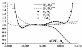
Figure 4a: IP bandwidth of the traditional NLC Final Focus. Normalized beta functions and normalized
