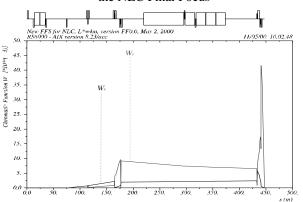
Figure 6b: Horizontal and vertical chromaticity through the New Final Focus
