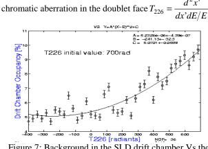
Figure 7: Background in the SLD drift chamber Vs the chromatic aberration  $T_{226}$
