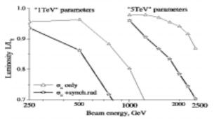
Figure 11: Luminosity Vs beam energy for the new FF, bend field optimized at each energy, with and without synchrotron radiation. The "1TeV" parameters correspond to Tab.1, the "5TeV" set corresponds to [4] with:  $\gamma \epsilon_{x/y} = 50/1 \cdot 10^{-8} \text{m}, \beta^*_{x/y} = 9.5/0.14 \text{mm}, \sigma_E = 0.2\%,$  $\sigma_{x/y}(2.5 \text{TeV/Beam}) = 31/0.54 \text{nm}.$
