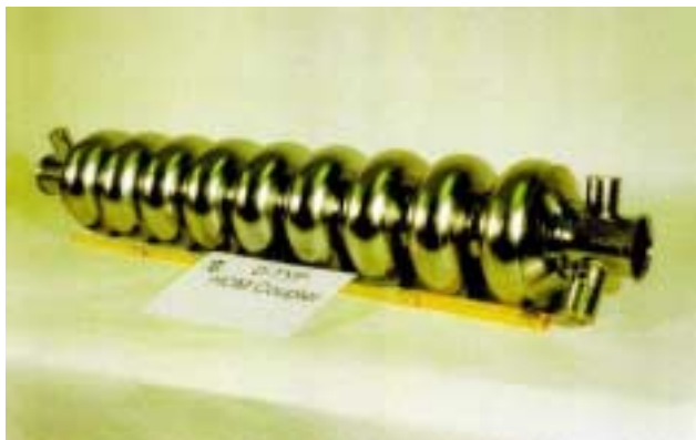
Fig. 1: The 9-cell TESLA Niobium cavity
